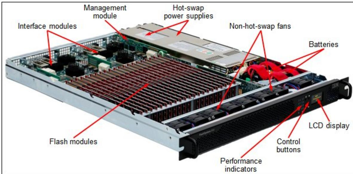
Figure 2. Internal view of the FlashSystem unit
